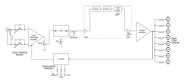
Figure 8-13. VPD-6830-DLY240 Block Diagram
